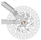
5. Install 2 stop pins and cap nuts onto the gear hub shaft from the both sides, and tighten them with a 19 mm wrench. (Tightening torque: 40-45N.m)
